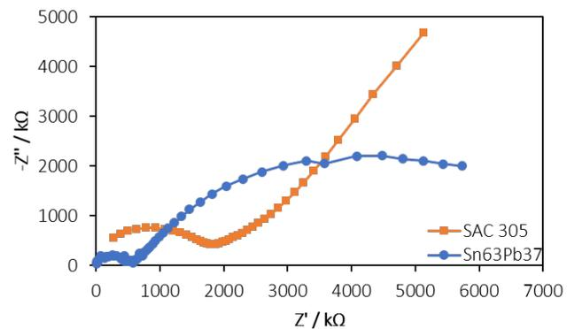
Fig. 5 EIS spectra for two solder pastes with different alloys: SAC305 and Sn63Pb37
