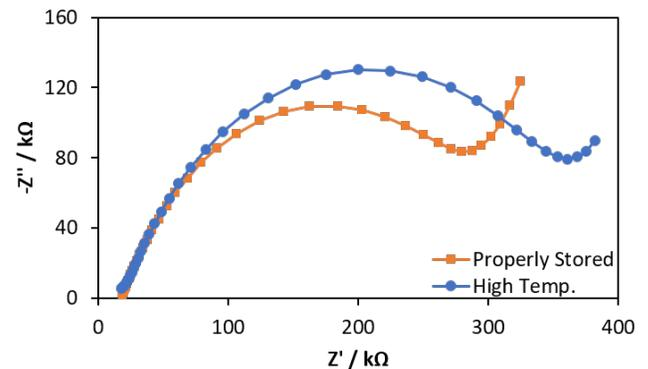
Fig. 4 EIS spectra for solder pastes properly stored vs. stored at high temperature
