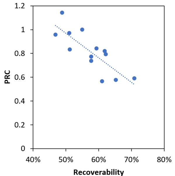
*Fig. 2 Correlation between the time constants and % recoverability of solder paste*
