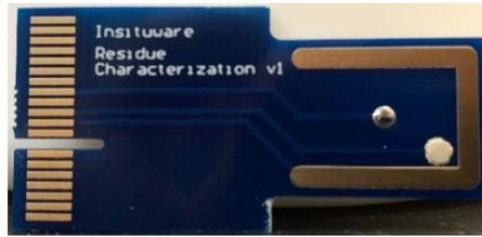
Figure 1. Three-electrode probe configuration used for LSV measurements
