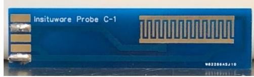
Figure 4. The two-electrode probe configuration used for the EIS measurements in this study.
