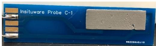
Figure 5. The probe covered with solder paste for EIS measurements.
